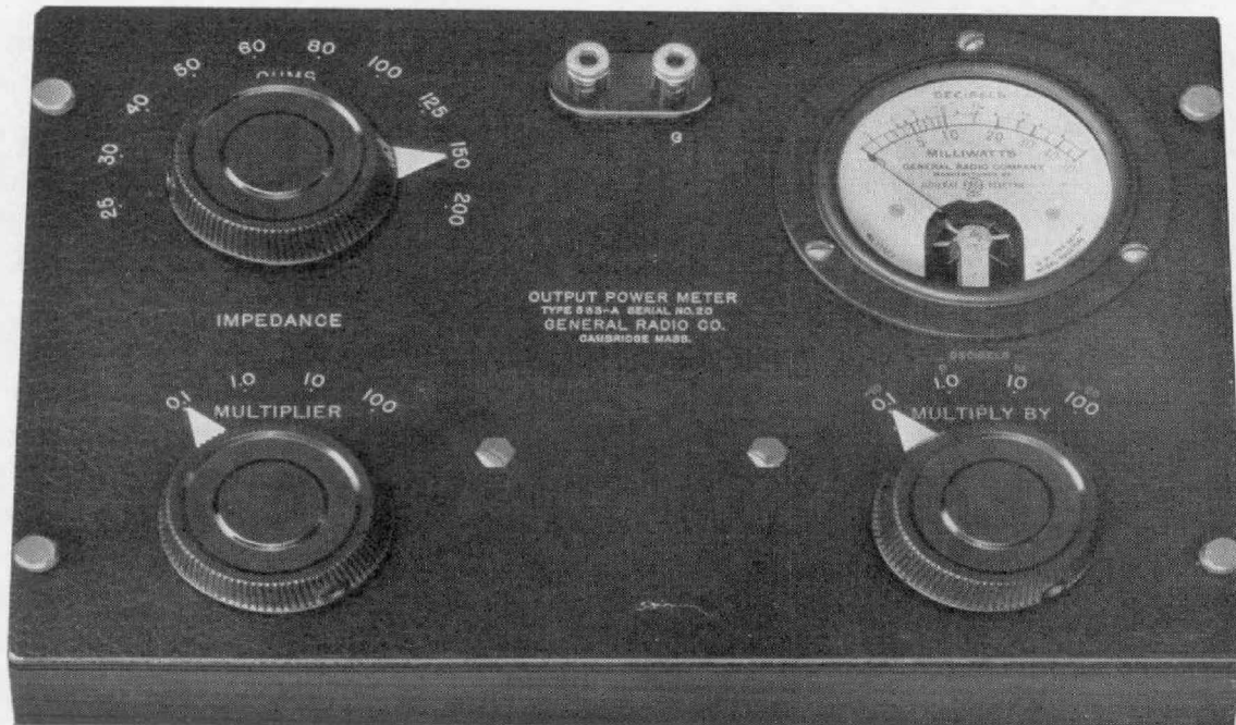
FIGURE 1. Panel view of a TYPE 583-A Output Power Meter, showing the available impedance settings and the meter scale
